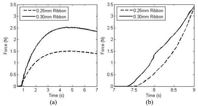
Fig. 2. Abaqus simulation results of the (a) required actuation force and (b) approximate jaw force for a 0.25- and 0.30-mm-thick ribbon.
