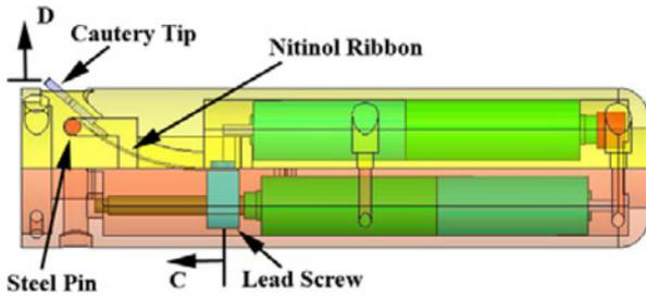
Fig. 4. Side view of CAD model illustrating the components of the cautery payload half of the robot.
