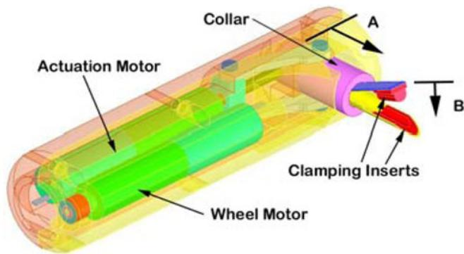
Fig. 1. Isometric view of CAD model illustrating the components of the clamping payload half of the robot. The control board, battery, and other wheel motor are located in the other half of the robot (not shown).
