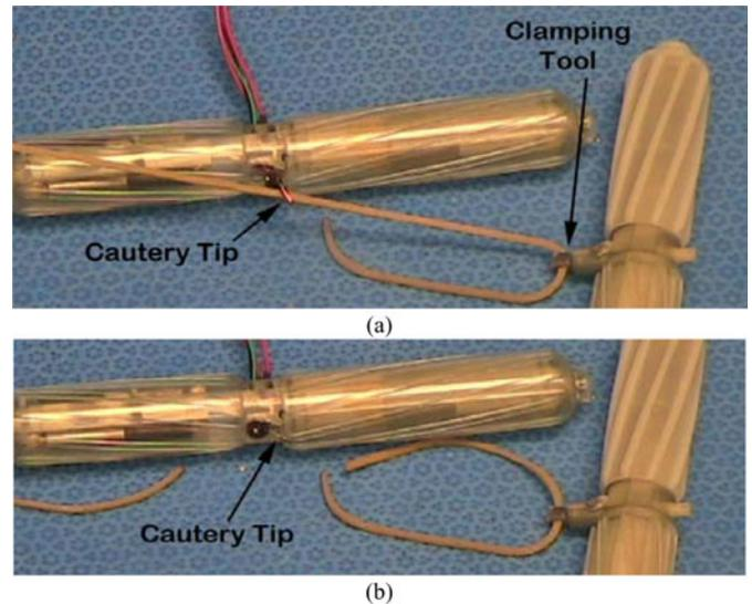
Fig. 7. (a) Laboratory experiments showing a “stretch and dissect” demonstration with multiple robots. (b) After the rubber band is dissected, the cautery tip is retracted.
