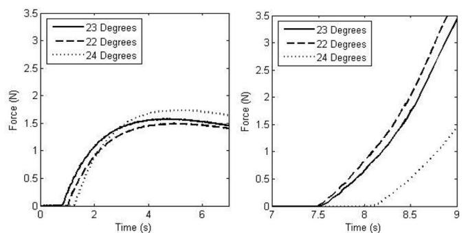
Fig. 3. Abaqus simulation results of the (a) required actuation force and (b) approximate jaw force for a 22°, 23°, and 24° ribbon profile angle.
