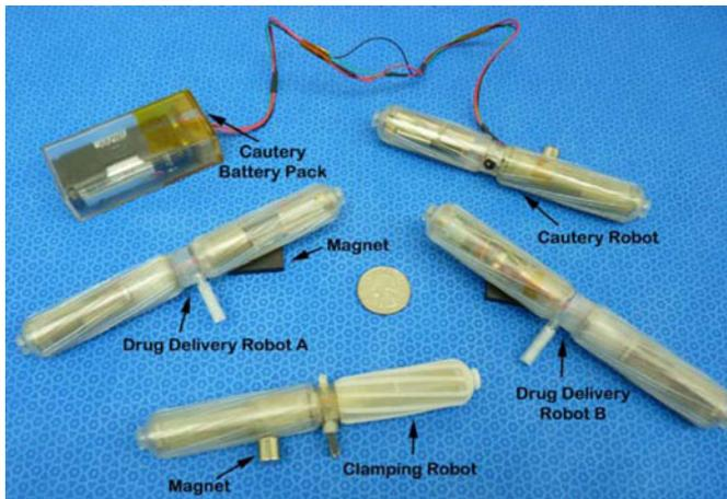
Fig. 6. Wireless mobile robots prior to insertion.
