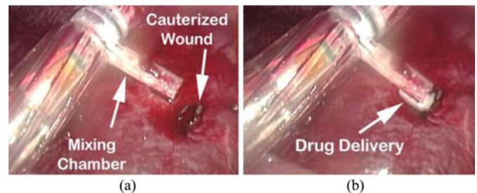
Fig. 10. *In vivo* images of (a) the liquid delivery robot approaching an injured area of the spleen, and (b) delivering a white liquid directly into a wound.
