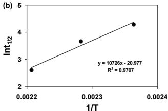
Figure 4. (a) Time dependence of the reduced grafted layer thickness  $(H/2R_{\rm g})$  at 150, 165, and 180 °C for D125K. (b) Arrhenius plot for grafting kinetics of D125K where  $t_{1/2}$  is the annealing time required to reach half of the final grafted amount. The activation energy  $(E_a)$ calculated from the plot is  $89 \pm 16$  kJ/mol.
