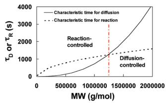
**Figure 9.** Characteristic times  $\tau_D$  and  $\tau_R$  in Kramer's model as a function of molecular weight. The crossing of these two curves denotes a critical molecular weight above which the grafting will become diffusion-controlled.
