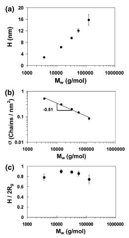
Figure 2. (a) Grafted layer thickness (H) as a function of telechelic molecular weight  $(M_w)$ . (b) Surface density  $(\sigma)$  as a function of telechelic molecular weight  $(M_w)$ . (c) Reduced grafted layer thickness  $(H/2R_{\rm g})$  as a function of telechelic molecular weight.
