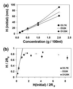
Figure 1. (a) Thickness of spin-coated films as a function of solution concentration for D3.7K, D32K, and D125K. (b) Reduced grafted layer thickness  $H/2R_g$  as a function of reduced initial film thickness.
