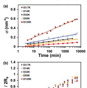
**Figure 3.** (a) Evolution of surface density  $(\sigma)$  with annealing time. (b) Time dependence of reduced grafted layer thickness  $(H/2R_{\rm g})$  for all of samples.
