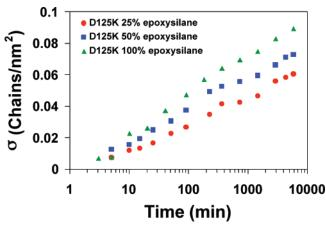
**Figure 6.** Time dependence of surface density for mixed silane layers with nominal epoxy surface density of 6/nm<sup>2</sup>, 3/nm<sup>2</sup>, and 1.5/nm<sup>2</sup>.
