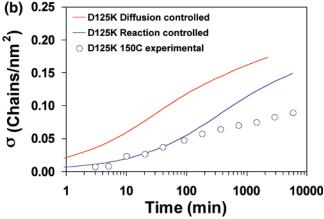
Figure 7. (a) Comparison of the kinetics curves (solid curves) calculated by Kramer's model assuming a diffusion-controlled mechanism with experimental data for D32K (black), D55K (blue), and D125K (red). (b) Fitting of a reaction-controlled mechanism model to the experimental data for D125K annealed at 150 °C. As a comparison, the theoretical prediction for a diffusion-controlled process is also shown in the plot.
