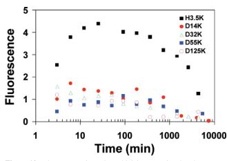
Figure 10. Fluorescence intensity, which is proportional to the amount of singly bound chains in the grafted layer, as a function of grafting time for samples with varying molecular weight.
