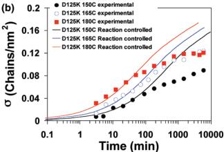
**Figure 8.** (a) Fitting of the kinetics curves to Kramer's model assuming reaction-controlled mechanism. Note that the same rate constant  $k_{\rm f}$  is used in all fits. (b) Fitting of the kinetics curves to Kramer's model assuming a reaction-controlled for varying grafting temperatures.
