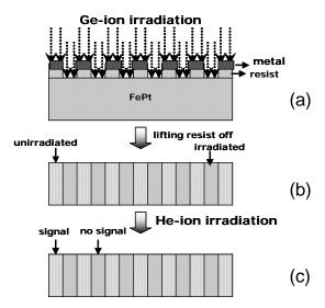
**Figure 5.** Schematic diagram of fabrication for patterned media by using ion irradiation. (a) Ge-ion irradiation is first performed, (b) resist and metals are removed and (c) He-ion irradiation is performed. The areas exposed to Ge-ion irradiation show no magnetic signal, but the rest
