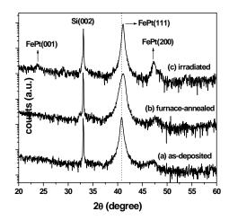
**Figure 2.** X-ray  $\theta$ -2 $\theta$  scans of (a) the as-deposited FePt film, (b) the unirradiated FePt film annealed in a vacuum furnace at 230 °C for 10 h, (c) the FePt film irradiated at a beam current of 1.25  $\mu$ A/cm<sup>2</sup> with a dose of 2.4x10<sup>16</sup> ions/cm<sup>2</sup>. (The dash line is used to indicate peak shift).
