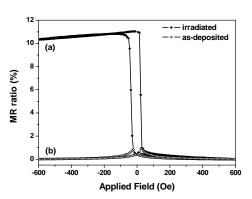
**Figure 8.** MR curves of (a) irradiated and (b) as-deposited spin valve samples. The irradiation fluence is  $1.91 \times 10^{16}$  ions/cm<sup>2</sup>.
