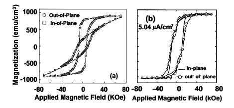
**Figure 6.** Magnetization curves for the sample (a) annealed at 550 °C for 300 sec by RTA method and (b) irradiated by using 2 MeV He-ions with current density of  $5.04 \,\mu\text{A/cm}^2$  for 360 secs
