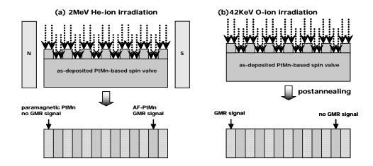
**Figure 9.** Schematic diagrams of magnetic patterning for PtMn-based spin valves by using (a) 2MeV He-ion irradiation and (b) 42 keV O-ion irradiation. The areas exposed to He ions in (a) show a high exchange field and GMR. The areas exposed to O-ion irradiation show no GMR.
