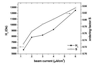
**Figure 3.** Dependence of coercivity  $H_c$  and ordering factor S on beam current for the samples irradiated at an ion dose of  $2.4x10^{16}$  ions/cm<sup>2</sup>.
