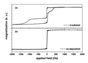
**Figure 7.** Hysteresis loops of (a) irradiated and (b) as-deposited spin valves. The irradiation fluence is  $1.91 \times 10^{16}$  ions/cm<sup>2</sup>.
