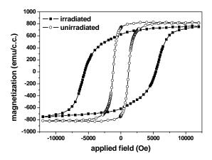
**Figure 1.** Hysteresis loops of irradiated and unirradiated FePt films. The He-irradiation was performed at a beam current of 1.25  $\mu$ A/cm<sup>2</sup> with an ion dose of 2.4x10<sup>16</sup> ions/cm<sup>2</sup>. The unirradiated FePt film was annealed in a furnace at 230 °C for 10 h.
