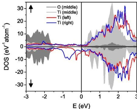
FIG. 2. (Color online) Local DOS in a Fe/BaTiO<sub>3</sub>/Fe ( $m=4$ ) tunnel junction as a function of energy. The O<sub>2</sub> and Ti DOS in the middle TiO<sub>2</sub> monolayer are shown by the shaded area. The polarization is assumed to be pointing to the right, as in Fig. 1(b).
