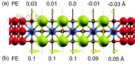
FIG. 1. (Color online) Atomic structure of a Fe/BaTiO<sub>3</sub>/Fe(001) tunnel junction. Arrows show displacements of Ti atoms with respect to O atoms within each TiO<sub>2</sub> monolayer for (a) paraelectric (PE) and (b) ferroelectric (FE) BaTiO<sub>3</sub>.
