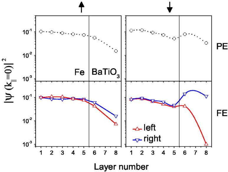
FIG. 3. (Color online) Majority-(left) and minority-spin (right) probability densities  $|\psi|^2$  for the state at  $\mathbf{k}_{\parallel}=0$  with the lowest decay rate ( $\Delta_5$ ) for paraelectric (top) and ferroelectric (bottom) states of a Fe/BaTiO<sub>3</sub>/Fe MFTJ at the Fermi energy. The results are obtained using VASP for a  $m=4$  BaTiO<sub>3</sub> barrier layer. Within BaTiO<sub>3</sub>  $|\psi|^2$  is displayed on Ti atoms.
