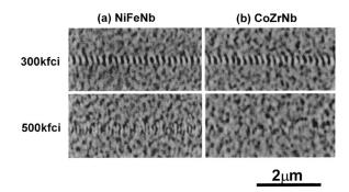
FIG. 2. MFM images of written tracks of 300 and 500 kfci for media with (a) NiFeNb and (b) CoZrNb SULs.
