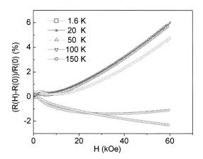
FIG. 2. High-field transverse MR, defined as  $(R_H - R_0)/R_0$ , at five different temperatures for single-grain size  $CrO_2$  sample with current parallel to the c axis geometry.
