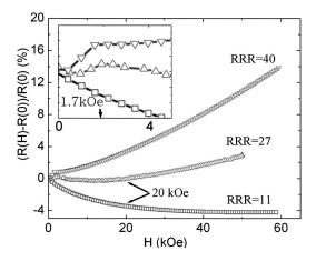
FIG. 3. Transverse MR vs applied magnetic field of grains aligned  $CrO_2$  films with different residual resistance ratios (RRR= $R_{273\,\mathrm{K}}/R_{4.2\,\mathrm{K}}$ ) measured with current parallel to c axis geometry. Inset shows the magnified low-field part of MR curves for the samples.
