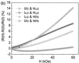
FIG. 4. Longitudinal and transverse MR for the current perpendicular and parallel to the c axis direction at low temperature (1.6 K) of (a) multigrain sample with the RRR value about 40 and (b) FIB milled single-grain sample.
