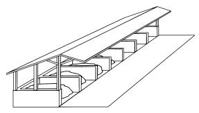
Figure 3. Roofed composting unit (high investment option).
