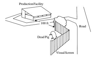
Figure 1. Carcass storage area for rendering pick up.
