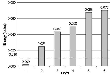
Fig. 3. Average energy consumption per node to revoke a compromised sensor in the 1000-node sensor network. The column value is also not the real average energy consumption  $e_v$  of the DistRev scheme but the value of  $2e_{\Delta_c}$ .
