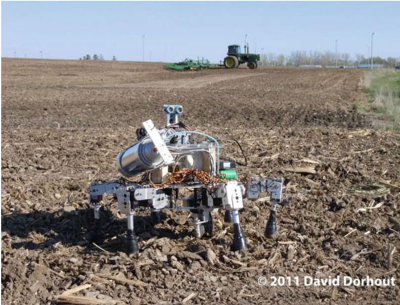
**Figure 5.** Prospero, the robot that plants and manages crops fields of the future. (Reprinted with permission from Dorhout R&D LLC (<http://dorhoutrd.com>))
