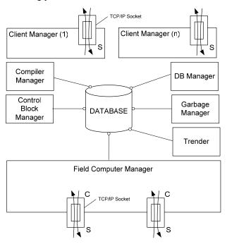
Figure 4: EMCS Application Server Software Components
