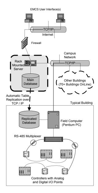
Figure 1: UNL EMCS Application Architecture
