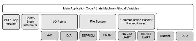
Figure 6: Controller Software Module Layering Scheme
