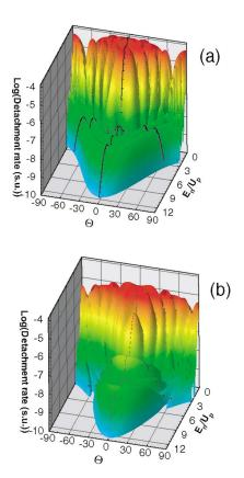
FIG. 2 (color online). Photoelectron ADs for (a) H<sup>-</sup> and (b) F<sup>-</sup> for the same laser parameters as in Fig. 1. The solid curves parallel to the  $\theta$  axis mark the ADs at the onset of the plateaus, i.e., at  $E_n = 3.8U_p$  (n = 28) for the s state and  $E_n = 4.37U_p$  (n = 31) for the p state. The first open ATD channel is  $n_0 = 10$ .
