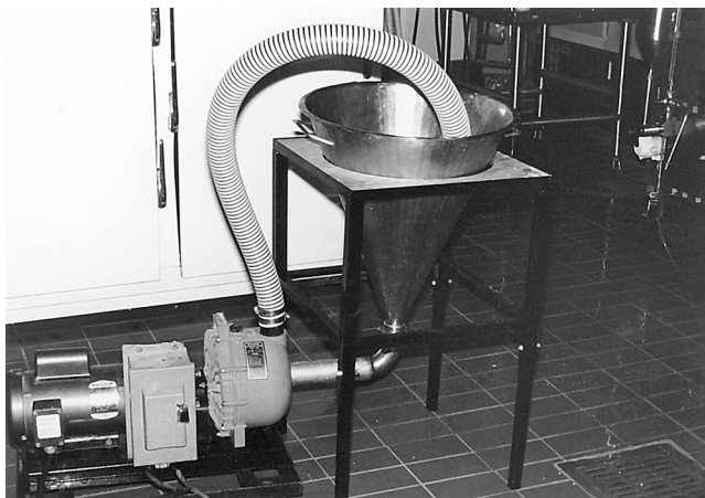
Figure 1—Recirculating system with hopper, pump, and wire reinforced, flexible hose.
