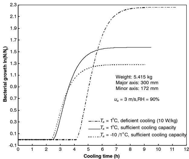
Figure 12. Predicted histories of bacterial growth of *Lactobacillus plantarum* at the center of cooked hams during air-blast cooling at different air temperatures ( $u_a$  = air velocity,  $T_a$  = air temperature, and RH = air relative humidity).
