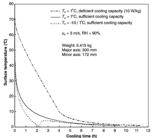
Figure 10. Predicted histories of surface temperature of cooked hams during air-blast cooling at different air temperatures ( $u_a$  = air velocity,  $T_a$  = air temperature, and RH = air relative humidity).
