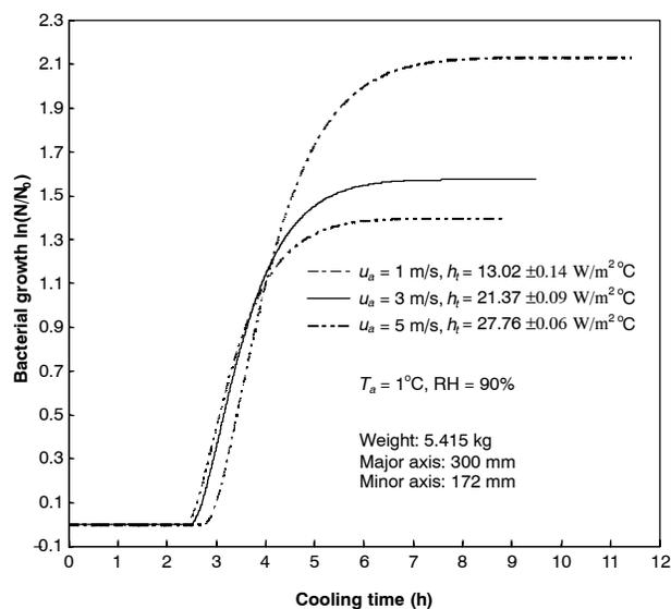
Figure 7. Predicted histories of bacterial growth of *Lactobacillus plantarum* at the center of cooked hams during air-blast cooling at different air velocities ( $u_a$  = air velocity,  $T_a$  = air temperature, RH = air relative humidity, and  $h_t$  = total surface heat transfer coefficient).
