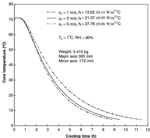
Figure 6. Predicted histories of core temperature of cooked hams during air-blast cooling at different air velocities ( $u_a$  = air velocity,  $T_a$  = air temperature, RH = air relative humidity, and  $h_t$  = total surface heat transfer coefficient).
