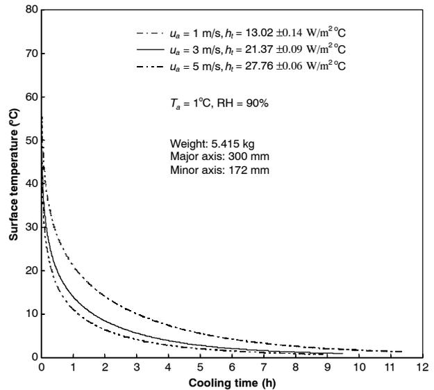
**Figure 5. Predicted histories of surface temperature of cooked hams during air-blast cooling at different air velocities ( $u_a$  = air velocity,  $T_a$  = air temperature, RH = air relative humidity, and  $h_t$  = total surface heat transfer coefficient).**
