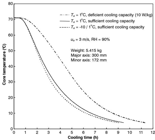
Figure 11. Predicted histories of core temperature of cooked hams during air-blast cooling at different air temperatures ( $u_a$  = air velocity,  $T_a$  = air temperature, and RH = air relative humidity).
