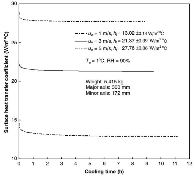
**Figure 4. Predicted histories of surface heat transfer coefficient during air-blast cooling at different air velocities ( $u_a$  = air velocity,  $T_a$  = air temperature, RH = air relative humidity, and  $h_t$  = total surface heat transfer coefficient).**
