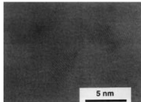
Fig. 2. High-resolution TEM image of  $\text{Co}_{57}\text{Pt}_{43}:\text{C}$  film.
