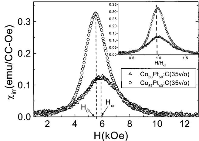
Fig. 3. The differential of DCD curves ( $\chi_{irr}$ ) for Co<sub>50</sub>Pt<sub>50</sub>:C and Co<sub>57</sub>Pt<sub>43</sub>:C films. The inset is normalized by remanence coercivity  $H_{cr}$ .
