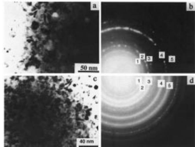
Fig. 1. (a) Bright field image and (b) electron diffraction pattern of sample  $\text{Co}_{50}\text{Pt}_{50}:\text{C}$ . (c) bright field image and (d) electron diffraction pattern of sample  $\text{Co}_{57}\text{Pt}_{43}:\text{C}$ . The indices for the rings are: 1 (001), 2 (110), 3 (111), 4 (202), 5 (311).
