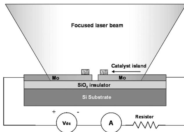
FIG. 1. Schematic diagram of electrical-field-directed laser-assisted CVD system.
