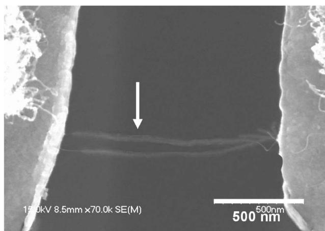
FIG. 3. SEM micrograph of two SWNTs bridging the electrodes synthesized by a focused CO<sub>2</sub> laser beam with a beam size of 340 μm in diameter.
