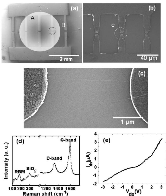
FIG. 2. (a) SEM micrograph of patterned Mo electrodes. Circle “A” is the typical unfocused 2 mm CO<sub>2</sub> laser beam irradiated on the substrate, while circle “B” is the typical focused laser beam with beam size of 340 μm using a 10 cm ZnSe lens. (b) Magnified electrode pairs inside circle B shown in (a). (c) SEM micrograph of two SWNTs bridging the electrodes inside circle “C” shown in (b). (d) Raman spectroscopy of SWNTs shown in (c). (e) *I*-*V* curve of the SWNTs shown in (c).
