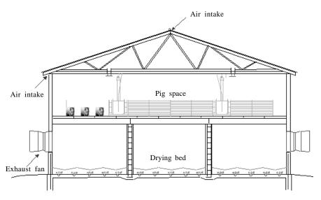
Figure 2. Cross-section view of commercial version of High-Rise<sup>TM</sup> finishing facility.
