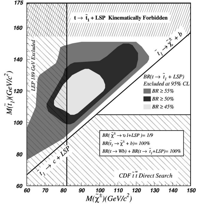
FIG. 3. Top into top squark plus LSP branching ratio limits as a function of top squark and chargino masses for a LSP mass of 20  $\text{GeV}/c^2$ .
