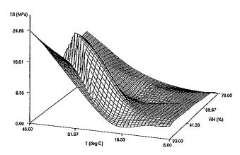
Figure 2-Plot of TS values of wheat gluten films with respect to conditioning RH and T.
