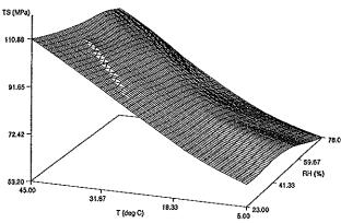
Figure 3-Plot of TS values of MC films with respect to conditioning RH and T.
