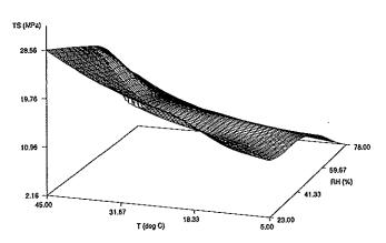
Figure 1-Plot of TS values of CZ films with respect to conditioning RH and T.
