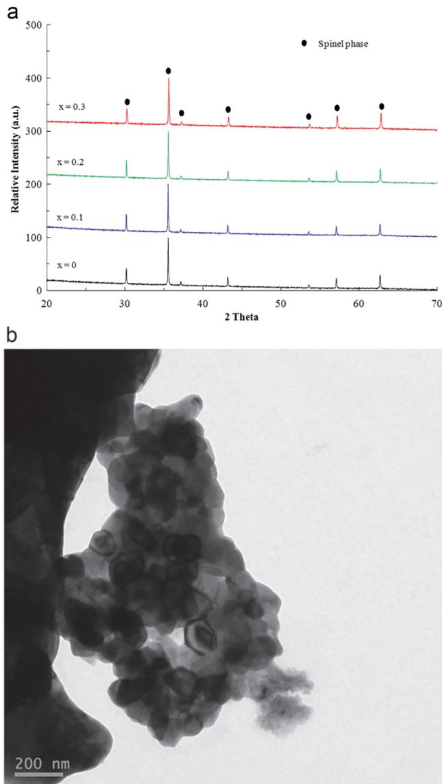
**Figure 2.** (a) X-ray diffraction spectra of calcined  $\text{CoZn}_x\text{Fe}_{2-x}\text{O}_4$  ( $x = 0, 0.1, 0.2,$  and  $0.3$ ); (b) Bright-field TEM image of the calcined  $\text{CoFe}_2\text{O}_4$ .
