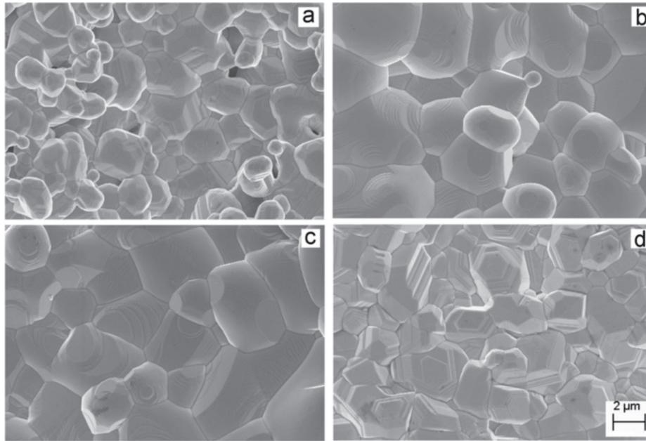
Figure 4. SEM micrographs of (a)  $\text{CoFe}_2\text{O}_4$ , (b)  $\text{CoFe}_{1.9}\text{Zn}_{0.1}\text{O}_4$ , (c)  $\text{CoFe}_{1.8}\text{Zn}_{0.2}\text{O}_4$ , and (d)  $\text{CoFe}_{1.7}\text{Zn}_{0.3}\text{O}_4$ , sintered at  $1300^\circ\text{C}$  for 12 h.
