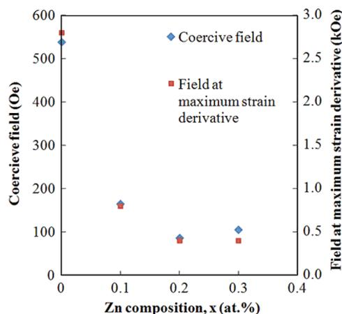
Figure 8. Correlation between coercive field ( $H_c$ ) and field required to attain maximum strain derivative ( $H$  in kOe) for  $\text{CoZn}_x\text{Fe}_{2-x}\text{O}_4$  ( $x = 0, 0.1, 0.2,$  and  $0.3$ ).
