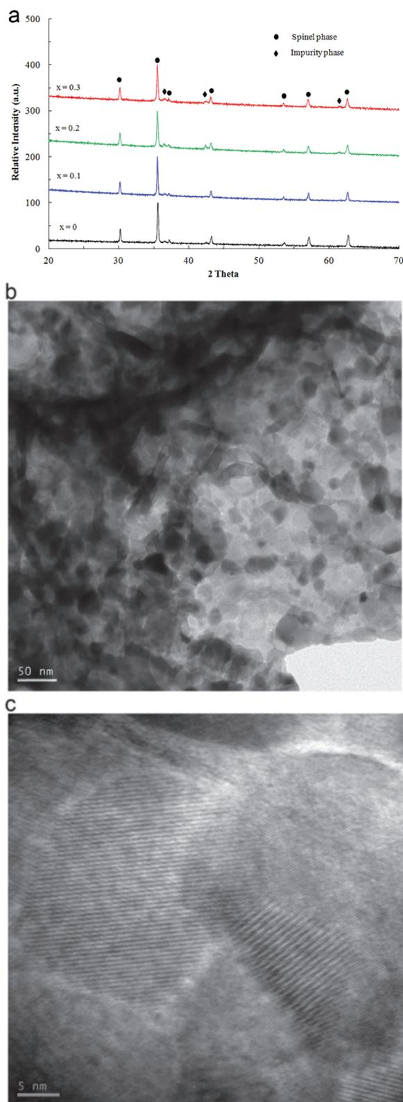
**Figure 1.** (a) X-ray diffraction spectra of as-prepared  $\text{CoZn}_x\text{Fe}_{2-x}\text{O}_4$  ( $x = 0, 0.1, 0.2,$  and  $0.3$ ) prepared by the auto-combustion method; (b) Bright-field and (c) High-resolution TEM image of as-prepared  $\text{CoFe}_2\text{O}_4$ .
