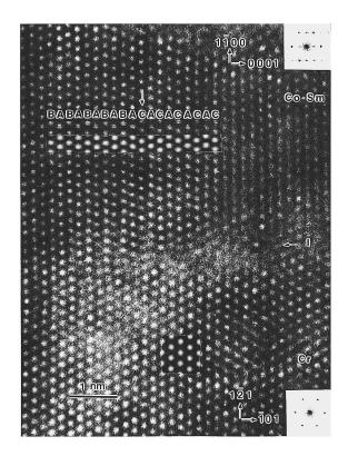
FIG. 2. Magnified interface region of Co-Sm on Cr underlayer. The stacking sequence in the Co-Sm film is well identified by the HREM image.
