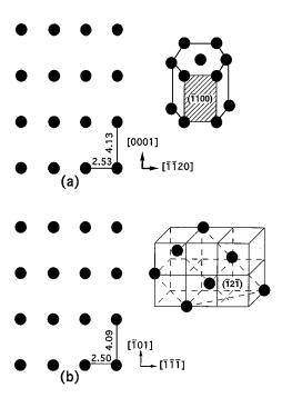
FIG. 3. Schematic illustration of atomic planes of (a) (1100) in Co-Sm of hexagonal unit cell with lattice parameters a = 0.253 nm, c = 0.413 nm. (b)  $(\bar{1}2\bar{1})$  in BCC Cr with lattice parameter a = 0.289 nm.
