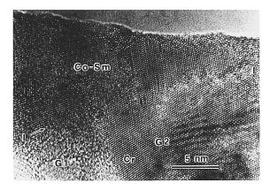
FIG. 1. HREM image of a cross-sectional Co-Sm film. A Cr grain is aligned on [111] zone axis while the Co-Sm crystallite is aligned on [1120] zone axis. The epitaxy is Cr (121)//Co-Sm (1100) and Cr [111]//[1120]. The interface is indicated by letter I.
