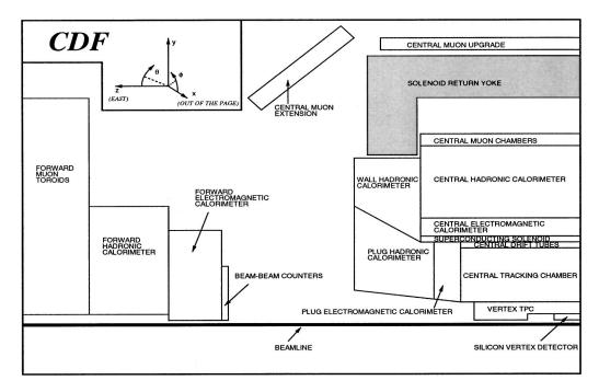
FIG. 2. One quarter of the Collider Detector at Fermilab. The major detector elements are indicated. The center of the detector is along the beam line to the far right.
