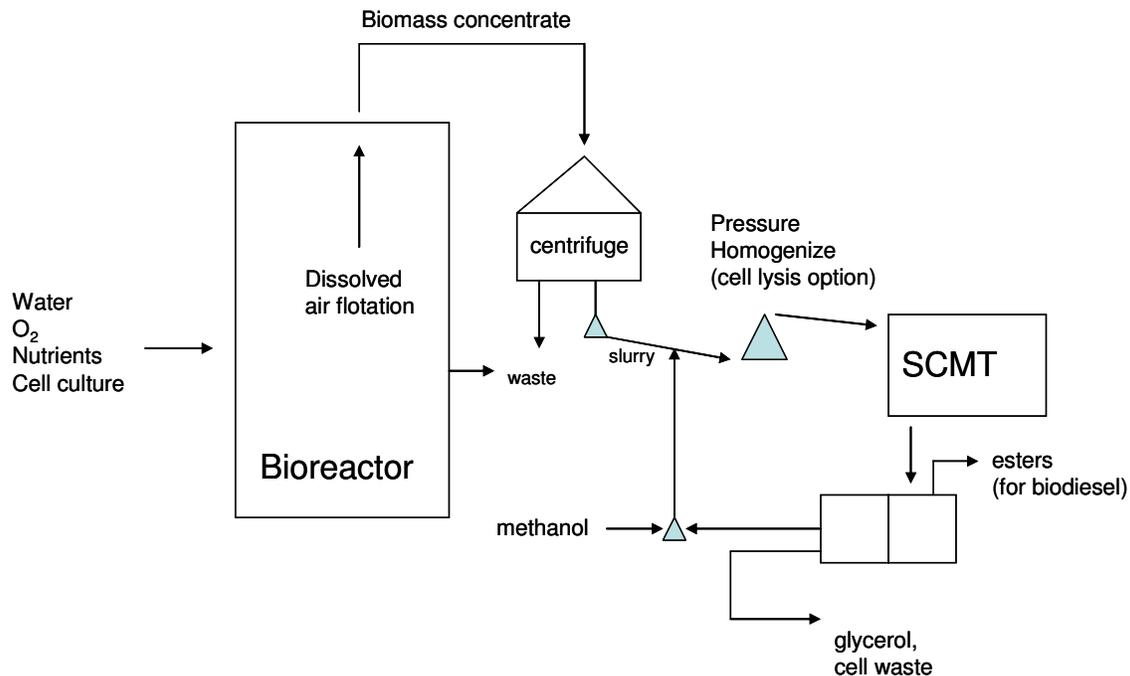
Figure 2. Candidate large-scale algal biodiesel process concept
