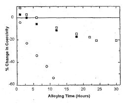
Fig. 4. Percent change in the coercivity of nanocomposited samples as defined in the text. 15-hour premilled samples are shown as squares and 2-hour premilled samples as circles. Aligned measurements are shown as solid symbols and unaligned measurements as open symbols.
