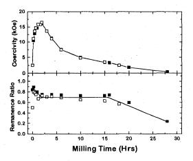
Fig 3: The remanence and coercivity as a function of milling time for SmCo<sub>5</sub> powders. Open symbols represent powders measured in the unaligned state, while solid symbols represent powders measured in an aligned state.
