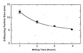
Fig. 2. Diffracting crystallite size of premilled  $SmCo_5$  as a function of milling time.
