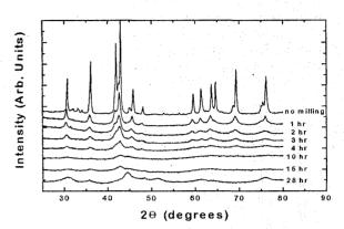
Fig. 1. The X-Ray diffraction spectra of premilled SmCo<sub>5</sub>.
