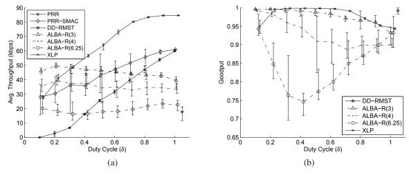
Fig. 8. (a) Average throughput and (b) average goodput vs. duty cycle for different values of  $\xi_{Th}$ .
