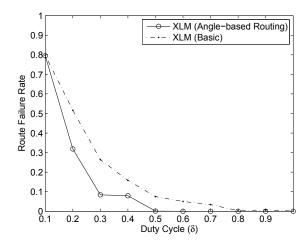
Fig. 5. Route Failure Rate for XLP with and without angle-based routing.
