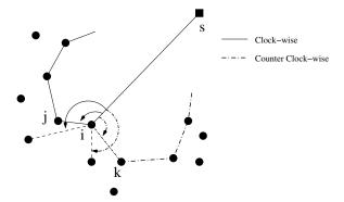
Fig. 2. Illustration of angle-based routing.
