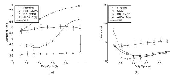
Fig. 10. (a) Average hop count, and (b) average latency vs. duty cycle for layered protocol suites and XLP.
