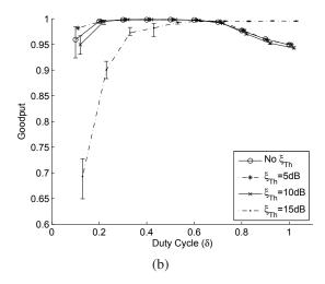
Fig. 6. (a) Average throughput and (b) average goodput vs. duty cycle for different values of  $\xi_{Th}$ .
