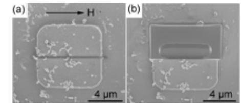
Fig. 2. (a) Double  $7\ \mu\text{m} \times 3.5\ \mu\text{m} \times 30\ \text{nm}$  bars patterned with focused ion beam (FIB) on the  $7\ \mu\text{m} \times 7\ \mu\text{m} \times 30\ \text{nm}$  Ni80Fe20 film with a gap of 50 nm between adjacent bars. (b) Single  $7\ \mu\text{m} \times 3.5\ \mu\text{m} \times 30\ \text{nm}$  bar after removing the top bar with FIB.
