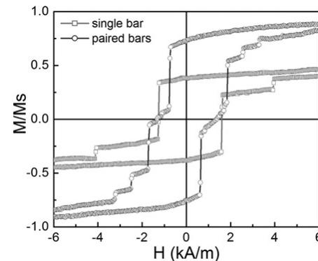
Fig. 3. Magnetic hysteresis loops of the single  $7\ \mu\text{m} \times 3.5\ \mu\text{m} \times 30\ \text{nm}$  Ni80Fe20 bar and same size paired bars with a gap of 50 nm obtained with a microcantilever torque magnetometer.
