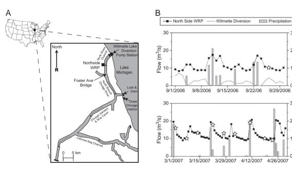
Fig. 1. (A) Map showing the Greater Chicago waterways, the North Side Water-Reclamation Plant (WRP) location, and the Foster Avenue Bridge North Shore Channel sampling location. (B) Flow from the North Side WRP and the Wilmette Pumping Station during the September 2006 and March-April 2007 sampling periods. [Open star symbols for the WRP flow indicate dates when water samples were collected; flow and precipitation data from Metropolitan Water Reclamation District (2010)].
