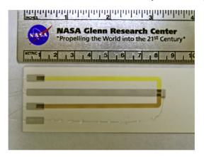
Fig. 2. Test sample composed of thin films of  $In_2O_3$ , Pt,  $N:In_2O_3$ , and a PtRh alloy wire on an alumina substrate.
