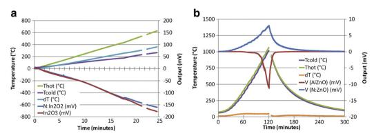
Fig. 3. Thermocouple output and temperatures vs. time for: (a) the  $ln_2O_3/N$ :  $ln_2O_3$  sample; and (b) the ZnO/AlZnO sample.
