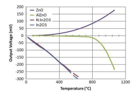
Fig. 5. Graphed thermoelectric output of the tested films vs. platinum referenced to 0  $^{\circ}\text{C}.$
