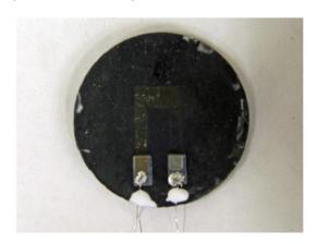
Fig. 4. EBC-CMC sample with ZnO vs. N:In<sub>2</sub>O<sub>3</sub> thermocouple.
