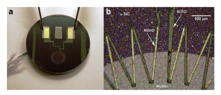
Fig. 1. Fine-lined AlZnO-N:ITO heat flux sensor on a 25 mm diameter  $\alpha$ -SiC disk: (a) during preliminary testing; and (b) a magnified view with films labeled.
