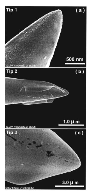
FIG. 1. SEM micrographs of the tungsten tips after laser irradiation in benzene solution (a) tip 1 with a curvature radius of 100 nm, aspect ratio of 3 under a laser fluence of 187 mJ/cm<sup>-2</sup>; (b) tip 2 with a curvature radius of 153 nm, aspect ratio of 3.5 under a laser fluence of 230 mJ/cm<sup>-2</sup>; and (c) tip 3 with a curvature radius of 480 nm, aspect ratio of 2 under a laser fluence of 230 mJ/cm<sup>-2</sup>.
