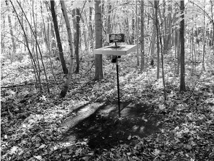
Figure 2. The Nuisance Bear Controller (NBC) positioned at a test site in central Minnesota. A simulated bird feeder sits above the square trigger plate that emits a shock when a bear or other animal moves the plate. A track plot has been cleared around the site to record the presence of animals visiting the NBC. Photo by M. Row.
