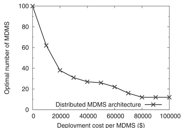
Fig. 8. Optimal number of MDMS versus deployment cost.
