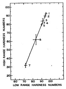
Fig. 4. Graph relating hardness values from the hard wheat (high) range of model II to values from the soft wheat (low) range. The samples used are: 1, durum sections exposed until an equlibrium condition was reached at 33% relative humidity (r.h.); 2, durum sections from wheat at 75% r.h.; 3, durum sections from wheat at 81% r.h.; 4, pure lead; 5, indium solder; 6, durum sections from a 93% r.h.; 7, polyethylene.
