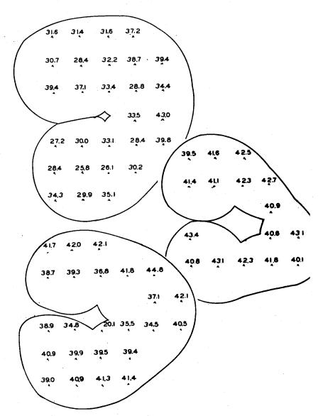
Fig. 5. Hardness values across sections of Ponca wheat, made with model I of the hardness tester. Top, section from germ end; bottom, middle of kernel; right, brush end.
