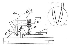
Fig. 2. Diagram of the converted Barcol Impressor. A, tester in lifted position; B, axis about which the tester swings; C, oak supports; D, oak platform which supports the sections to be tested; E, plane which contains the upper surface of the sections and the axis mentioned in B; F, penetrator; G, two-way movement stage.
