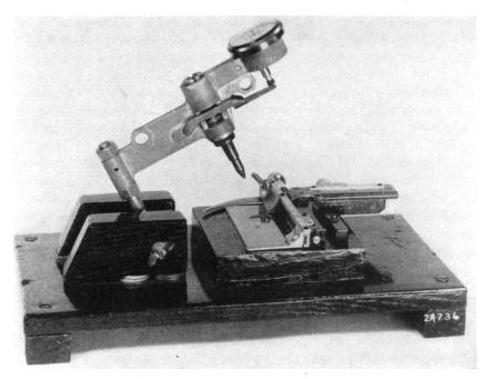
Fig. 1. The converted Barcol Impressor.
