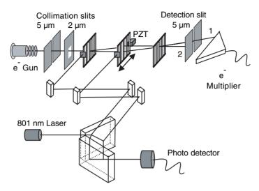
**Figure 1.** Sketch showing the experimental setup including the light interferometer used to measure the grating position (not to scale). Two slits are used to collimate the electron beam before it reaches the three-grating (100 nm periodicity) interferometer and an additional slit is used to select the interferometer output port (output ports 1 and 2 are indicated and 1 is selected in this example).
