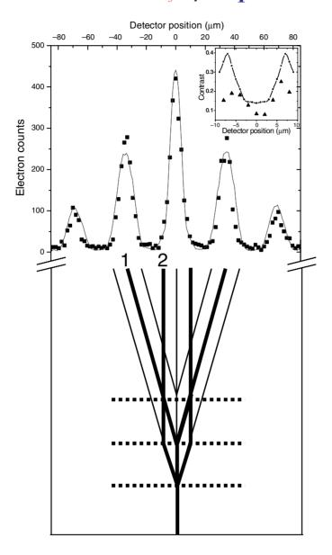
**Figure 3.** Electron diffraction through the interferometer at 10 keV. The solid line is the full path integral quantum mechanical calculation. Interferometer output ports are numbered 1 and 2. Contrast as a function of detector position for the zero order is shown in the inset (triangular data points). The solid line in the inset corresponds to a spline fit through the theoretical data points. The dip in contrast is a feature of a Mach–Zehnder interferometer.
