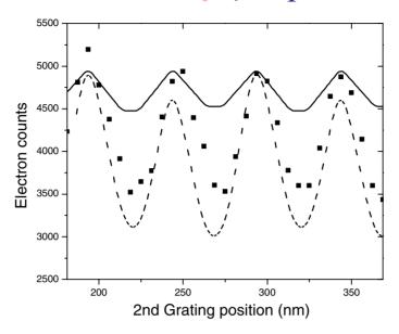
**Figure 4.** Experimental data comparison to theory. The result of the classical straight line path calculation is represented by the solid line. The result of the full path integral calculation is represented by the dashed line. Experimental data are represented by square dots. The contrast of our device exceeds the classical contrast by about three times, showing the quantum mechanical nature of our data.
