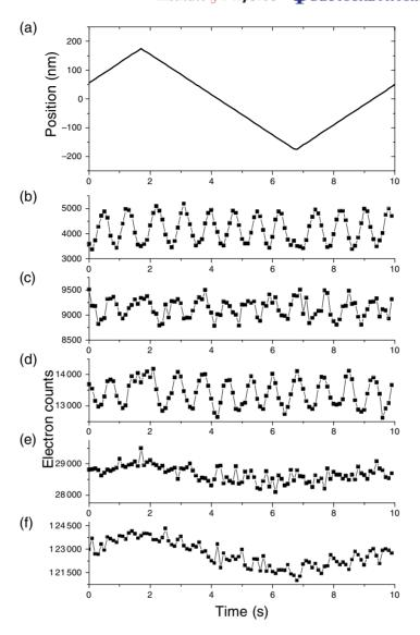
**Figure 2.** Electron interference data at output port 1. Figure 2(a) is the relative position of the second grating in nanometres. The experimental data are given for (b) 10 (c) 8 (d) 6 (e) 4 and (f) 2 keV. Note that for the vertical axis the zero is suppressed. The 10, 8, and 6 keV data show 50 nm periodicity fringes, while the 4 and 2 keV data do not show fringes.
