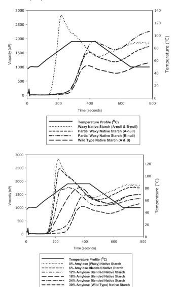
Fig. 2. Starch pasting properties of tetraploid durum wheat starches and starch blends.
