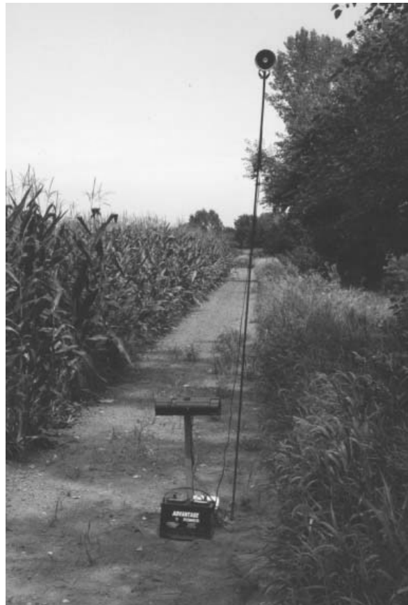
Figure 1. Infrared transmitting unit (left) and receiving unit (right) of the deer-activated bio-acoustic frightening device along the edge of a cornfield.
