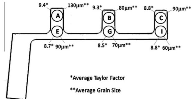
**Figure 1.** The initial average grain size and initial Taylor factor in the extruded magnesium AM30 alloy. The fatigue specimens were machined from sections A, B, C, E, G, and I as indicated in the cross-sectional view of the extruded alloy.
