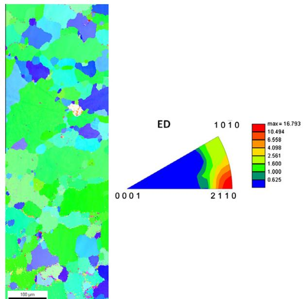
**Figure 2.** EBSD mapping showing the texture characteristics of section A in the extruded direction (ED).
