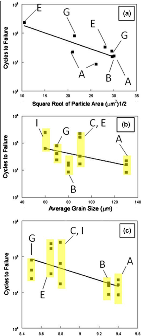
**Figure 4.** Number of cycles to failure vs. the square root of the particle area (a), average grain size (b), and average Taylor factor (c) for the magnesium AM30 alloy. The locations from the rail cross-section of the specimens are also shown.
