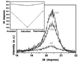
Figure 3 The  $\langle 110 \rangle$  diffraction peak at 20–21° of the ferroelectric copolymer vinylidene fluoride with trifluoroethylene P(VDF-TrFE): (a) annealed; (b) reannealed; (c) with water (saturated). Inset: reversibility of the bulk lattice parameter due to the process of absorption and desorption.
