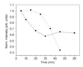
**Fig. 3.** Relative intensity of the P(VDF–TrFE 70:30) desorption peak at 150 K with respect to time after adsorption at 120 K, 3 ML ( $\blacksquare$ ) and 25 ML ( $\bullet$ ), respectively.
