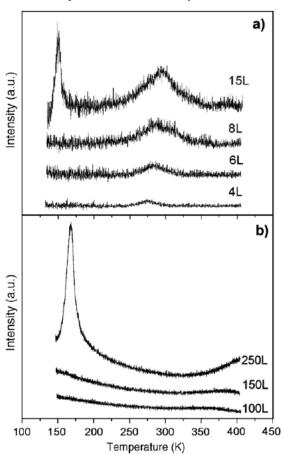
**Fig. 1.** Coverage dependent thermal desorption from a) 3 ML and b) 35 ML thick P(VDF–TrFE, 70:30) samples cooled to 125 K, and then exposed to water vapor. The broad peak at 280–300 K is the signature of the desorption of absorbed water, while the sharp peak at 150–160 K is surface ice, indicating that surface ice formation at roughly 15 L and 250 L on the 3 ML and 35 ML thick P(VDF–TrFE, 70:30) samples respectively.
