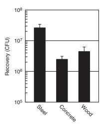
**Figure 1** Recovery from stainless steel inoculation control coupons, as well as concrete and wood positive control coupons by wipe sampling. Data are reported as mean recovered CFU  $\pm 1$  standard deviation, across all five tests. Each test consisted of three stainless steel, six concrete and six wood replicates, therefore n=15, 30 and 30, for stainless steel, concrete and wood, respectively.
