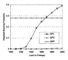
Fig. 4. Performance of the three grooming algorithms. Dedicated protection scheme is used with GPL and GPC. Fiber link availability is 99.9%.
