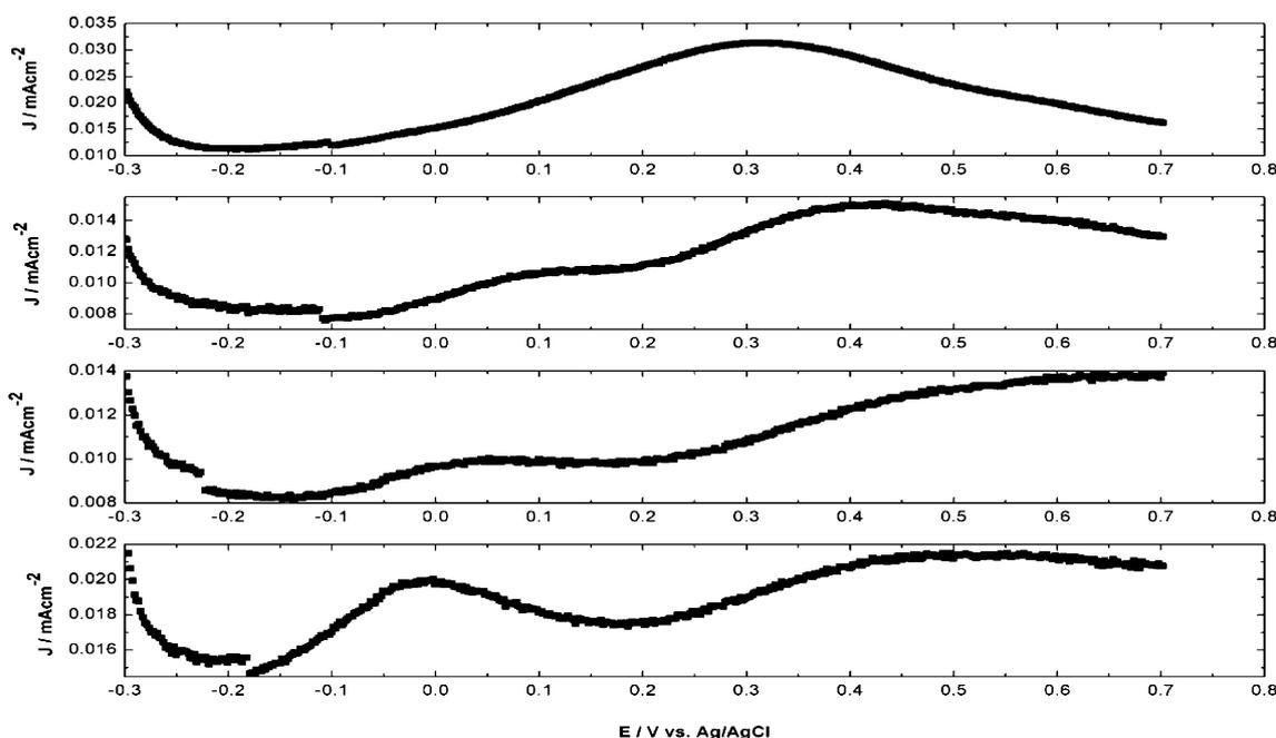
Fig. 4. Differential pulse voltammetry: (a) blank buffer, (b) 100 mM urea solution, (c) 1 mg/mL urease solution and (d) 100 mM urea-urease system at pH 8.3. Pulse height of 50 mV, pulse duration of 50 ms, step height of 2 mV, and step duration of 400 ms.
