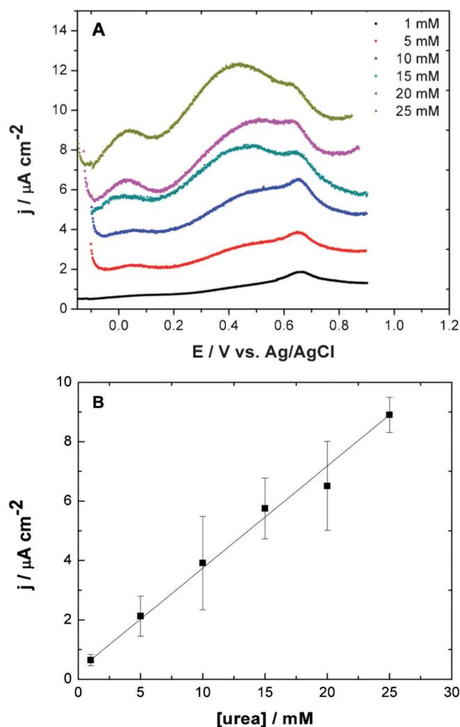
Fig. 5. (a). Differential pulse voltammetry of the ammonia oxidation for urea solutions of increasing concentration. Pulse height of 50 mV, pulse duration of 50 ms, step height of 2 mV, and step duration of 400 ms. (b). Calibration curve for the biosensor, with linear range from 1 mM to 25 mM and detection limit of 1.79 mM ( $S/N=3$ ), slope = 0.343  $\mu\text{A cm}^{-2}/\text{mM}$ . The data was obtained from (a).
