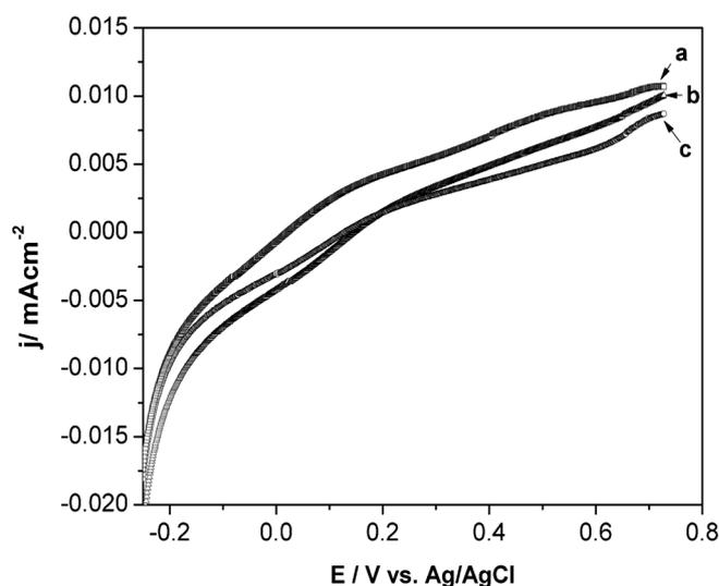
Fig. 6. Creatinine linear polarization: (a) 50 mM of creatinine, 10 mM of urea, and 0.5 mg/mL of urease in 100 mM PBS solution, (b) 50 mM of creatinine 100 mM PBS solution, (c) 50 mM of creatinine and 0.5 mg/mL of urease in 100 mM PBS solution. Scan rate of 5 mV/s.
