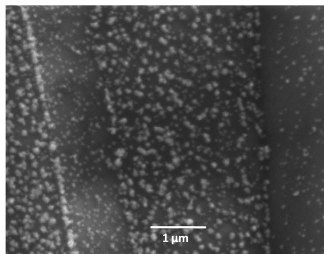
Fig. 2. Scanning electron microscopy image for the electrodeposited Pt nanoparticles at a boron doped diamond electrode, at  $20$  kV and  $20\times$  magnification.
