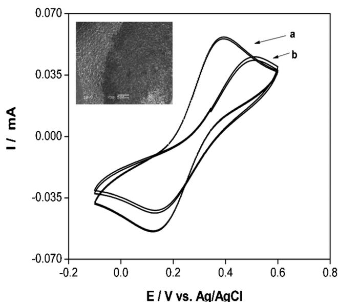
Fig. 1. Cyclic voltammograms of  $1$  mM  $\text{Fe}(\text{CN})_6^{3-/4-}$  in  $0.10$  M KCl at a boron doped diamond (BDD) electrode before and after the oxidation process at a scan rate of  $100$  mV/s. Inset: Scanning electron microscope image for the oxidized BDD electrode, at  $20$  kV and  $30\times$  magnification.
