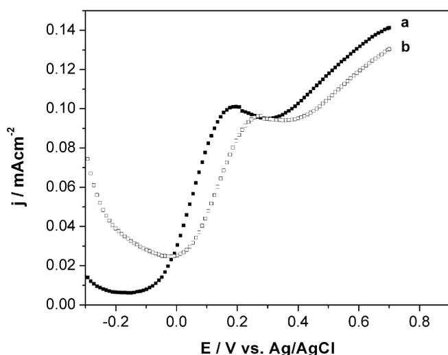
Fig. 3. Linear polarization of the ammonia oxidation at Pt nanoparticles at a boron doped diamond electrode in an ammonium sulfate solution in phosphate buffer solution at pH 7.4 and 8.3. Scan rate of 100 mV/s.
