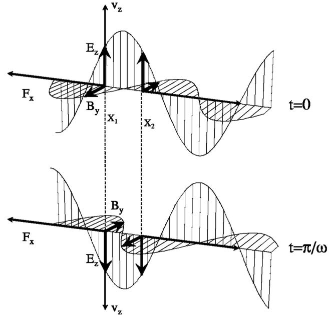
FIG. 2. Standing-wave fields. The electric ( $E_z$ ) and magnetic ( $B_y$ ) fields of a standing wave and the force ( $F_x$ ) on an electron with velocity ( $v_z$ ) at position  $x_1$  and  $x_2$  are given. An electron placed at  $x_1$  feels a Lorentz force in the same direction at times separated by half a light period, even though the fields have switched direction. This gives rise to a time-averaged potential from which electrons can diffract.
