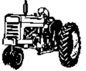
Tractor speeds should match surface conditions. Rough or uneven surfaces require reduced speeds. Be alert for rocks, holes, embankments or other hazards that can change the tractor's center of gravity.
