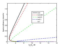
Fig. 2. Spectral efficiency vs.  $E_b/N_0$  in the Rayleigh channel with  $E\{|h|^2\}=\gamma=1.$   $B=10^5.$
