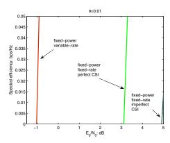
Fig. 4. Comparison of spectral efficiency;  $\bar{P}/N_0=10^4,\,\theta=0.01,$  and  $E\{|h|^2\}=\gamma=1.$
