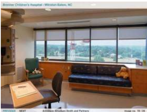
Figure 18-Woven shade cloth is more easily wiped clean or vacuumed and does not allow for the accumulation of as much contaminated dust.
