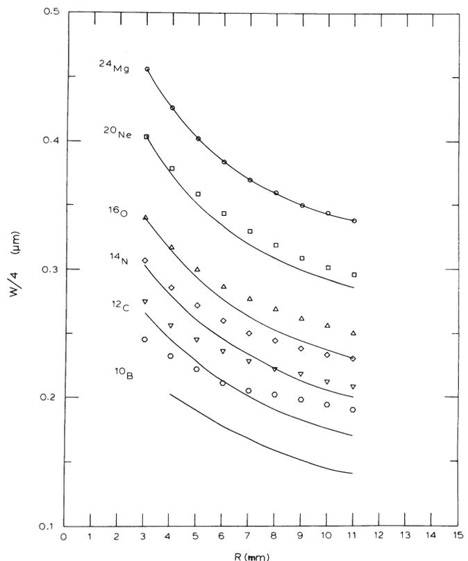
**Figure 1.** Track width  $W/4 \mu\text{m}$  vs residual range, of cosmic ray ions in G.5 emulsion. Light scattering parameters are fitted to the track of a  $^{24}\text{Mg}$  ion. When the width is calculated for lighter ions (curves) they depart increasingly from the measured width as  $Z$  decreases to  $^{10}\text{B}$  — (S. Behrnetz, private communication [1976]).
