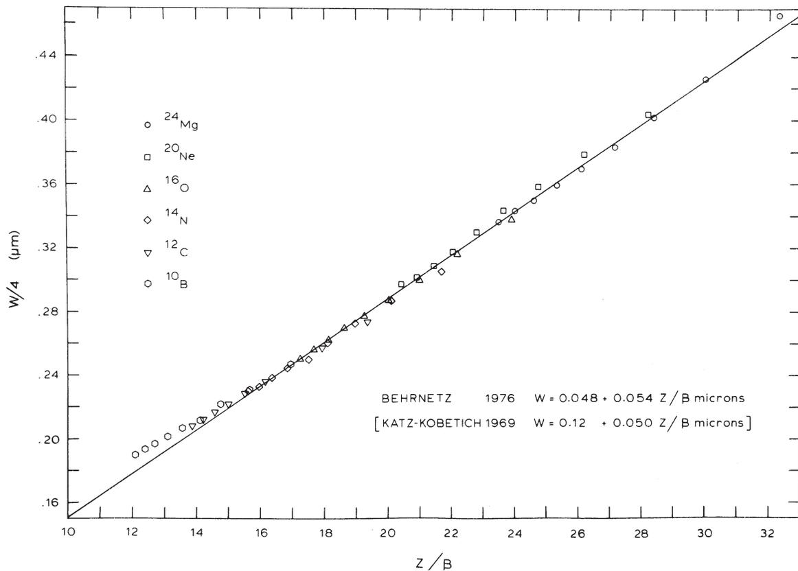
**Figure 2.** The data of Figure 1 are replotted as  $W/4 \mu\text{m}$  vs  $Z/\beta$ . A straight line is fitted to these data visually. The equation of that line is compared to an expression for the "visual width" of a heavy ion track, from theory, using values of  $E_0$  and  $P$  suggested for G.5 emulsion in 1969.
