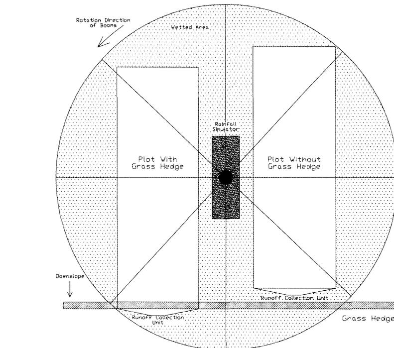
Figure 1. Plot diagram of a rainfall simulation site.
