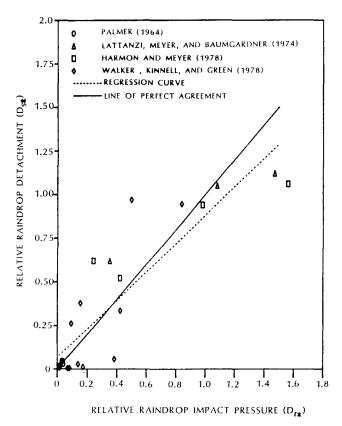
Fig. 3—Relative raindrop detachment vs. relative raindrop impact pressure.
