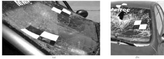
**Figure 3.** Vehicle damage, test no. WZ09-2: (a) System 2A, and (b) System 2B.
