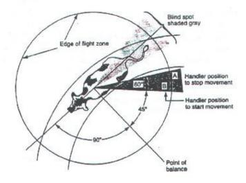
Diagram 2 - Handler movement pattern to keep cattle moving into a squeeze chute or restrainer
