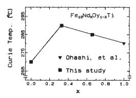
FIG. 4. Curie temperature vs composition for the Fe<sub>10</sub>Nd<sub>x</sub>Dy<sub>1-x</sub>Ti series.
