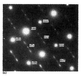
FIG. 2. Electron diffraction data for heat-treated Fe $_{10}$  DyTi. (a) shows fourfold rotation symmetry about [001]. In (b) the beam is along [100], and a modulation of about 12 Å along the c direction is seen.
