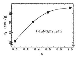
FIG. 5. Magnetization at H=8 kOe vs composition for the  $Fe_{10}Nd_xDy_{1-x}Ti$  series.
