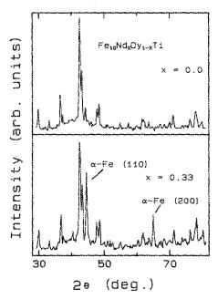
FIG. 1. X-ray diffraction patterns for x = 0.0 and 0.33 (CuK $\alpha$  radiation).
